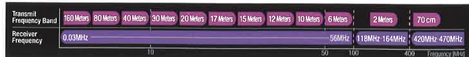
《Wide coverage from HF to UHF bands》 * Specified performance: Amateur bands only
